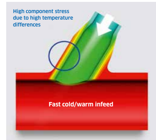
Fig. 1: Mechanical stresses caused by temperature changes.
